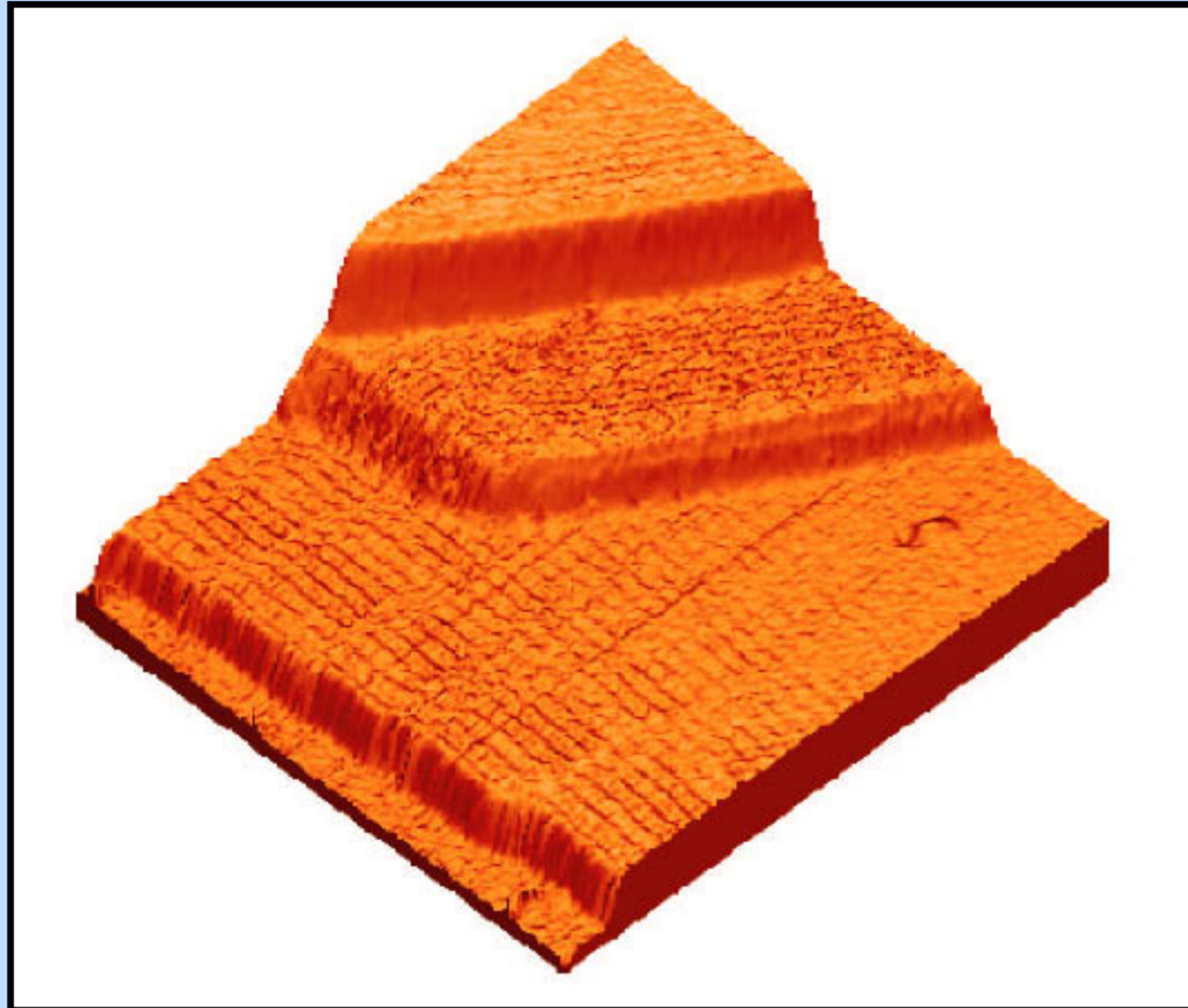
Figure 1. A STM image showing a 2-5 ML thick sodium island grown on graphite. Standing waves appear due to the quantum wells within the layers in the island. The scan size is 20 nm x 20 nm.
